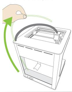
Remove the filament spool from the packaging and place it on the spool holder.
